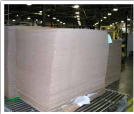
Figure 1. Twist warp of corrugated board due to fiber alignment problems
