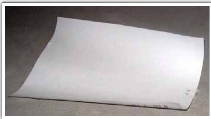
FIGURE 3. CURL AWAY FROM PRINTED SIDE OF LASER COPY PAPER DUE TO HIGH MOISTURE CONTENT.
