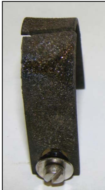
Cracked 2¼Cr-1 Mo sample
