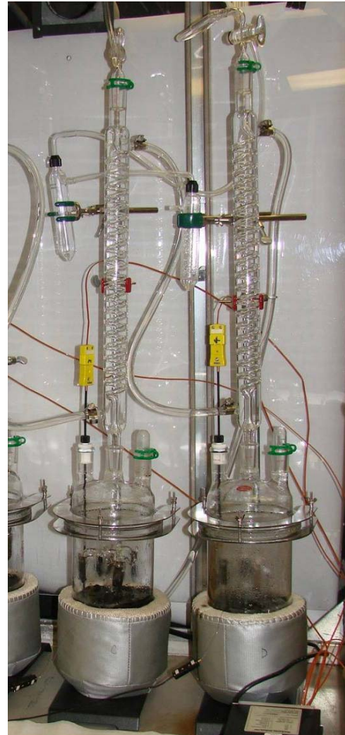
Two test systems used for pyrolysis oil corrosion tests
