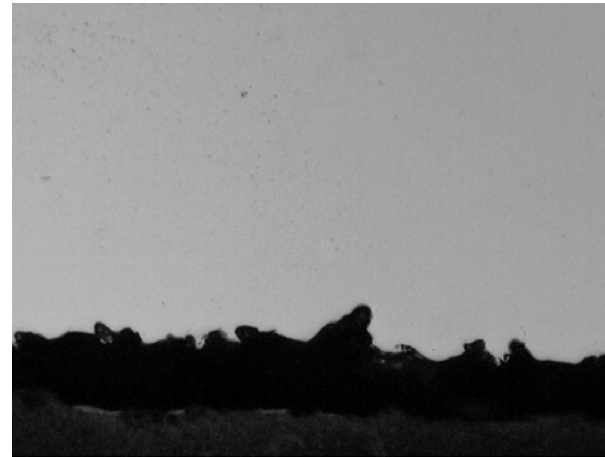
11-0016-04 316 0° I.D. 500x 10µm As polished
