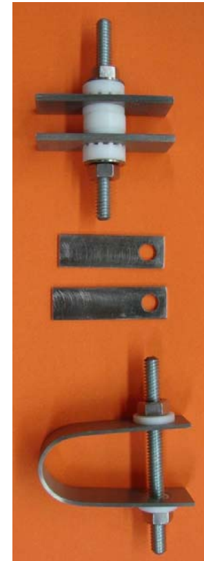
Samples used to assess localized, general and stress corrosion cracking
