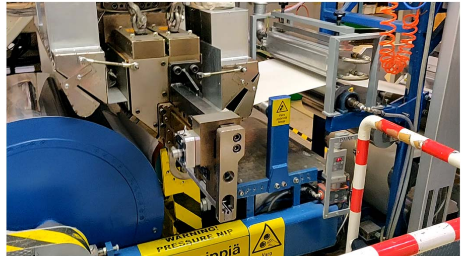
Pilot scale extrusion coater at Tampere University
