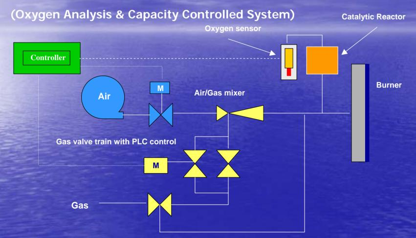
The Analyser is far more accurate than flow meters and measure the air gas ratio directly, flow meters try to quantify the air gas ratio but they do it indirectly and cannot automatically compensate
