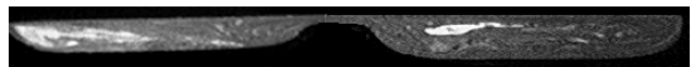
Figure 6. Channel cross sections for the ET extruder screw (9). The white regions are un-melted resin while the gray regions indicate molten and well-mixed resin.
