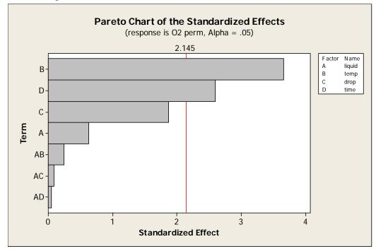
It is interesting to note that neither dropping the pouches nor the heat transfer mechanism inside the pouch had a significant impact on the test results.
