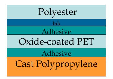
The commercial converter also prepared stand-up pouches with a flat-bottom gusset for evaluation. Barrier properties of the SiOx-coated PET were not compromised during adhesive laminating to form the rollstock, maintaining a value of  $0.3 \text{ cc/m}^2/\text{day}$ . However, during stand-up pouch forming the barrier properties of the three faces of the pouch (front, back and bottom gusset) were all somewhat compromised:
