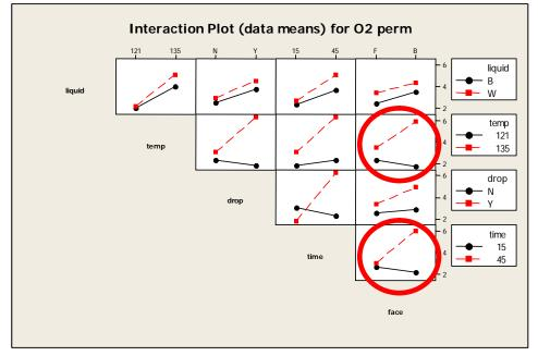
We then re-evaluated the DOE using our original four variables under investigation. In this case, we found two primary effects on oxygen barrier: the top one was retort temperature, the lesser one was retort time.
