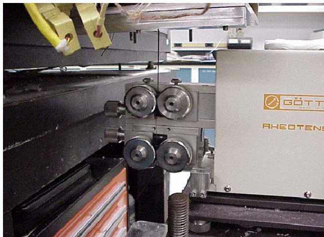
Figure – 12 Rheotens melt strength measurement. (Credit: Gottfert)
