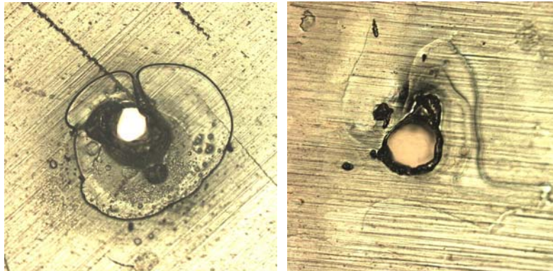
FIGURE 4 Delamination Areas on Both Sides of Foil PET Side at 100X LDPE Side at 100X
