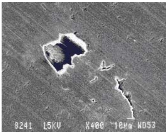
Pinhole from rolling Debris
