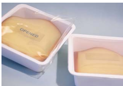
Figure 1. Oxygen indicator detecting leak.
