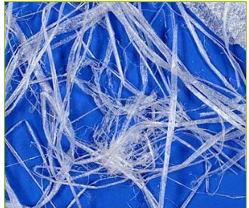
Streamers : Broad (>2mm) ribbons of polymer with a length from approx. 20mm
