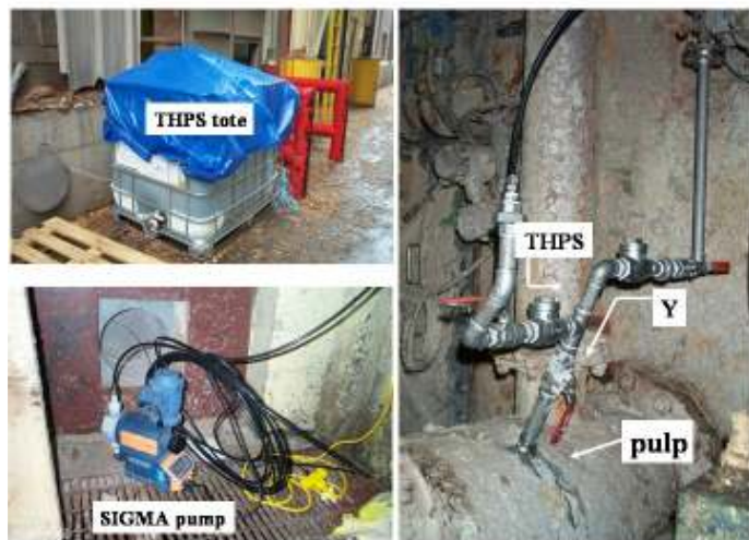
Fig. 3. Set-up for the “THPS + Y” bleaching mill trial.
