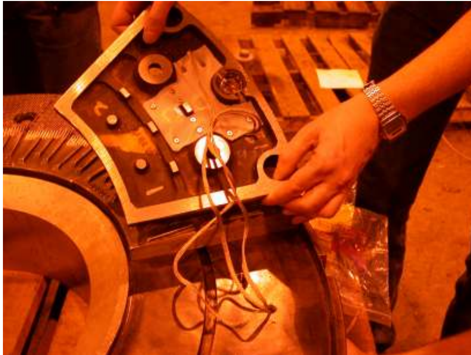
Installation of instrumented 36604 plate
