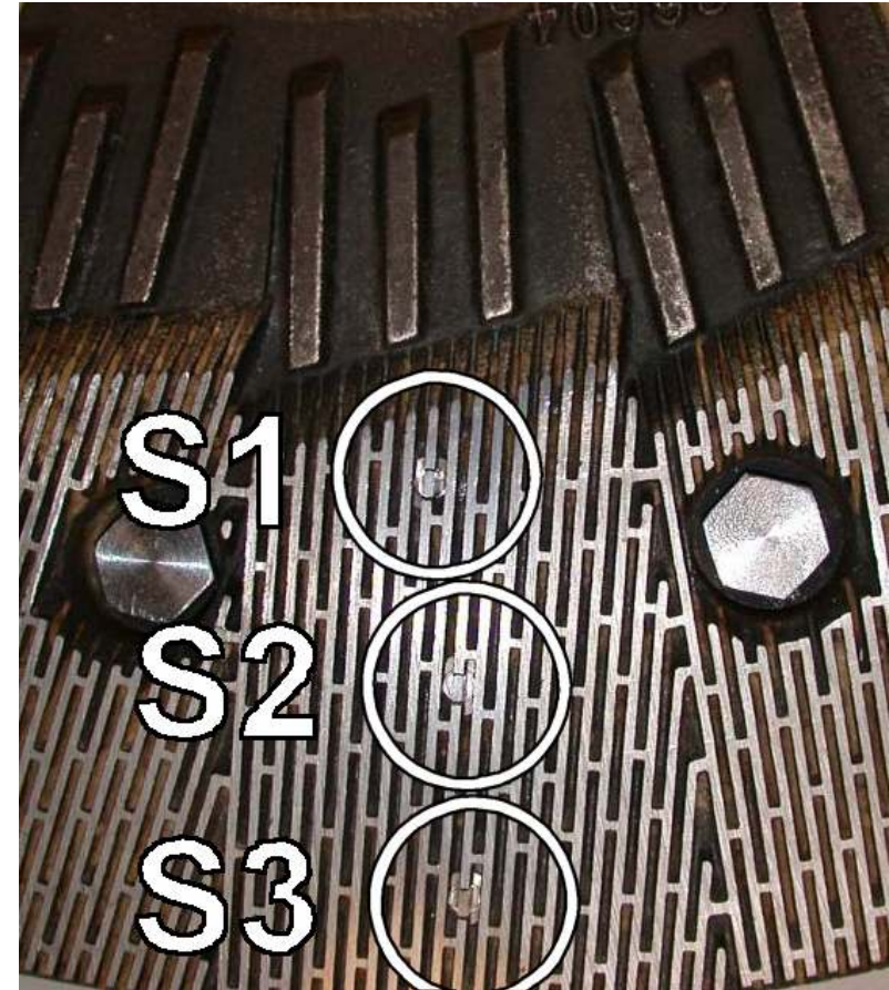
Identification of RFS in 36604 plate
