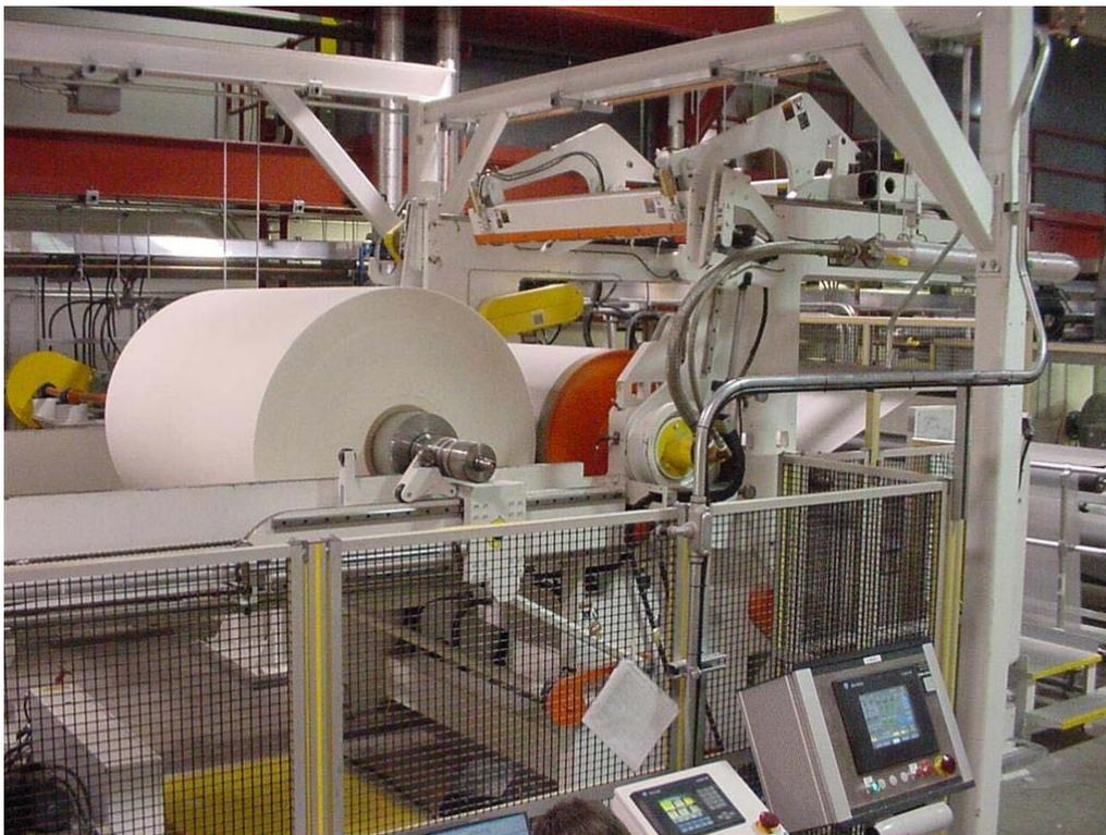
**Drum Winder on a Nonwoven Coating Line**
