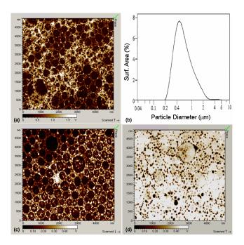
**Figure 1.** a.) Atomic force microcopy (AFM) image of a label-grade, water-based acrylic pressure sensitive adhesive film, b.) The particle size distribution for the adhesive in the latex, and AFM images for the film at c.) 3% and d.) 90% relative humidity.
