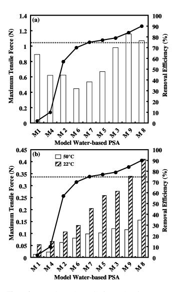
**Figure 3.** (a) Maximum dry tensile force values for the model water-based PSA films (21 °C and 50% RH). Superimposed are their removal efficiencies measured at 50 °C (solid dots). (b) Maximum tensile force values for the model water-based PSAs after soaking in water for 1 minute at 22 °C (solid bars) and 50 °C (striped bars). Reprinted with permission from Reference 4. Copyright 2007 American Chemical Society.
