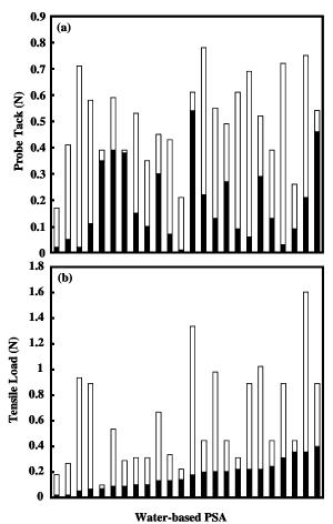
**Figure 2.** Measures of dry (longer bars) and wet (shorter bars) a.) Tack and b.) tensile force required to fail the films for 24 commercial water-based acrylic PSAs.
