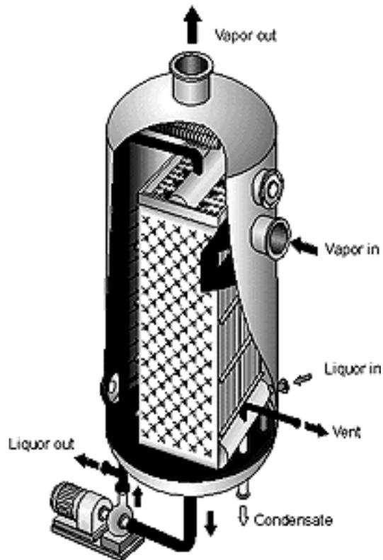
Following the distribution device, a thin film of liquor is established on the heating surfaces and flows downward back to the liquor sump while being partially evaporated. Heat-transfer rates are considerably better, especially at higher concentrations, when using falling film designs over rising film designs since the liquor falls turbulently over the heating surface. Any liquor preheating requirement is also efficiently accomplished in the falling film design.
