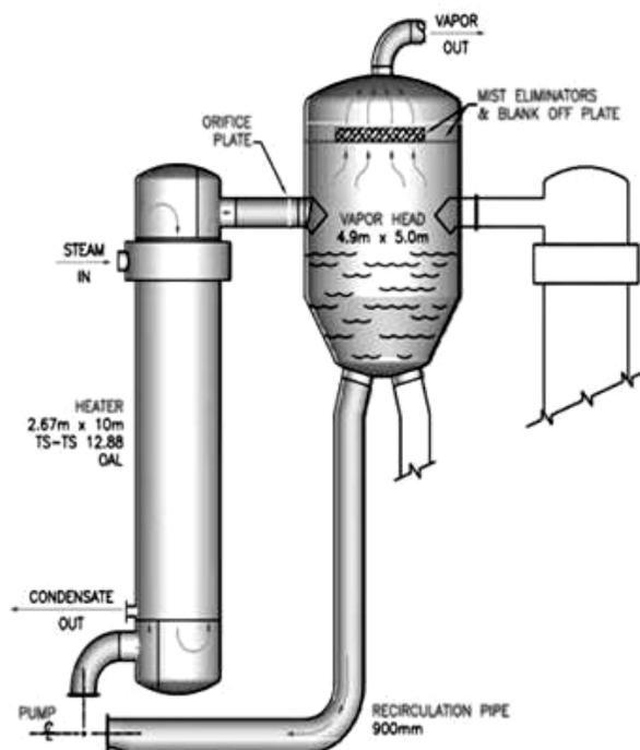
Liquor is heated in the heating element that is back-pressured to prevent boiling within the tubes. Boiling and evaporation occurs away from the heat transfer surface and only when the heated liquor enters the flash chamber
