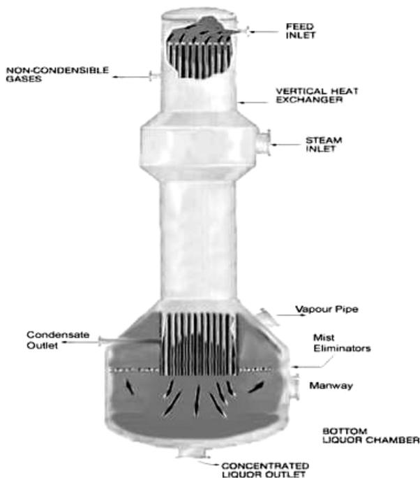
FF evaporators consist of a liquor sump from which a defined volume of liquor is continuously recirculated to the top of the heating element.
