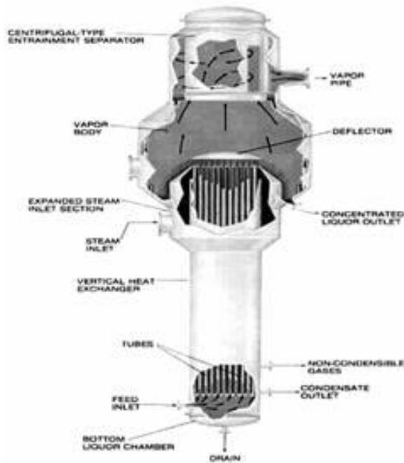
The heating element is a shell and tube heat exchanger using 2” OD tubes, typically 24ft. to 30 ft. long. Liquor is fed into the bottom liquor chamber and then into the tubes. It is heated with condensing steam on the outside of the tubes. The lower portion of the tubes is used to preheat the liquor to its boiling point. Evaporation then begins at that height within the tubes where the vapor pressure of the feed liquor equals the system pressure.
