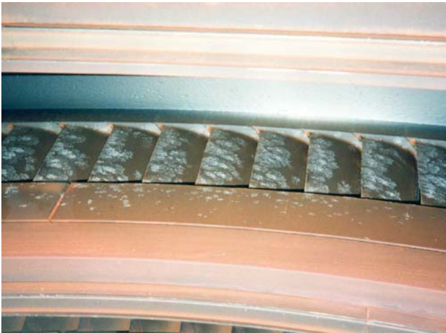
Figure 6 - Turbine Deposits Example
