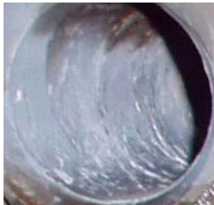
Figure 23 - Hardness in Generation Bank Tube
