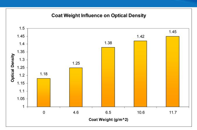
NPC coated papers printed at Kodak on the Versamark printer showed significant optical density increase as NPC coat weight increased
