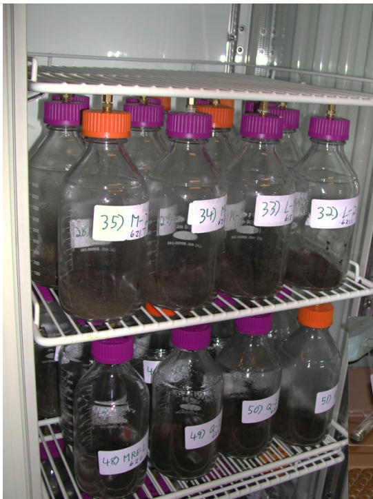
Composting vessels in incubator ( 52 \pm 1^\circ\text{C} )
