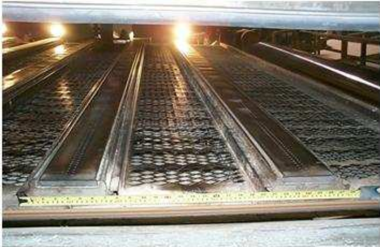
Before- slotted bars (wide spacing) and large screens
