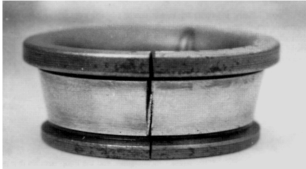
Figure 3. Cracked Bearing Inner Race (1). Courtesy Society of Tribologists and Lubrication Engineers.
