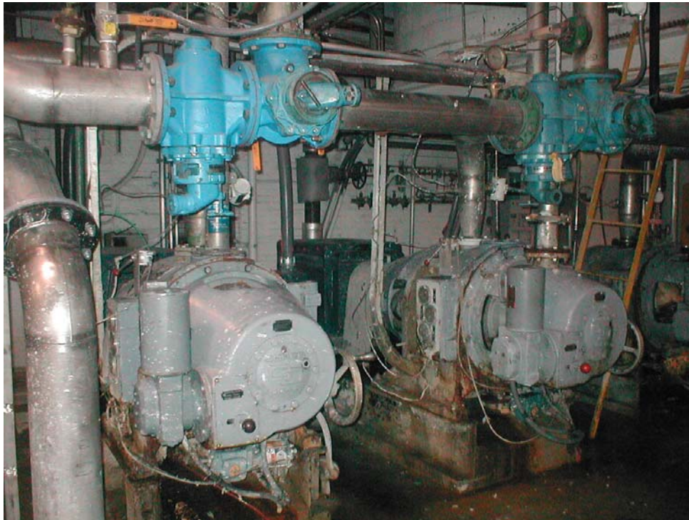
Photo 1. Refiners compared in Case History No. 1 (courtesy of Focus and Shawano Specialty Papers)
