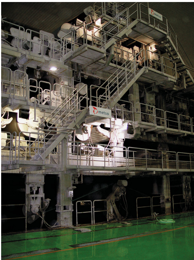
The Ningbo Xiaogang PM1 is the largest containerboard machine in the world.
