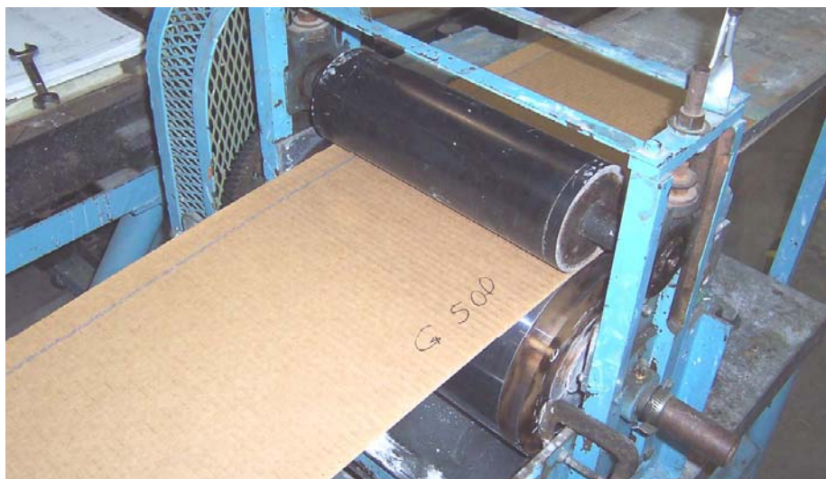
Figure 3. Corrugated board blank being sent through a double backing glue applicator nip to crush the board to a preset fraction of the original caliper.
