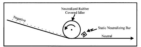
Figure 7 Static Bar Positioned to Neutralize Both Negative Charged Film and Positive Charged Idler Roll.
