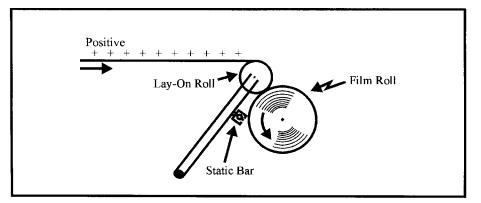
Figure 8 Static Neutralizing Bar Mounted on Lay-On Roll Support Arm to Neutralize Film Roll.
