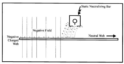
Figure 6 Field from Charged Film Web Attracts Opposite Polarity Ions from Static Bar, Neutralizing the Web.
