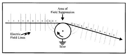
Figure 4 Example of Field Suppression Where Web Passes Over Metal Idler Roll.
