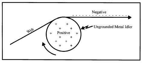
Figure 3 Tribocharging of Ungrounded Idler Roll and Film Web.
