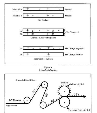
Figure 2 Cumulative Charges on Film Web Caused by Contact with Several Surfaces.
