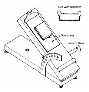
4.2.2.3 Means to level the instrument in two directions when the inclined plane is in its horizontal position.
