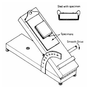
4.2.2.3 Means to level the instrument in two directions when the inclined plane is in its horizontal position.
