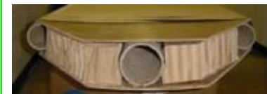
This cross-section shows the paperboard and paperboard tubes used in construction of the sailboard.
