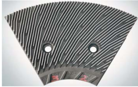
Figure 3 Curved-bar low intensity refiner filling
