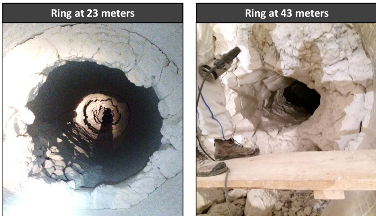
Figure 7. Rings form at 23 and 43 meters from the discharge end.
