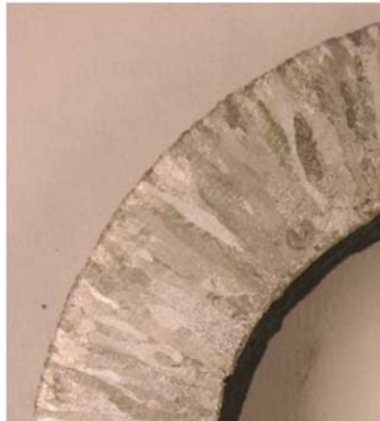
Figure 1: Grain macrostructure of cast corrosion resistant alloy.
