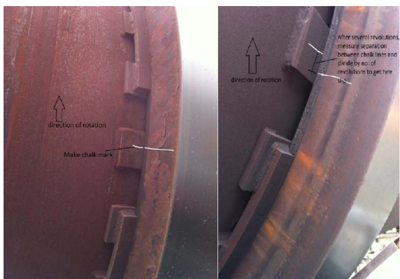
Figure 3 – Shows marking kiln components for creep (on left) & result after completing a rotation (on right).
