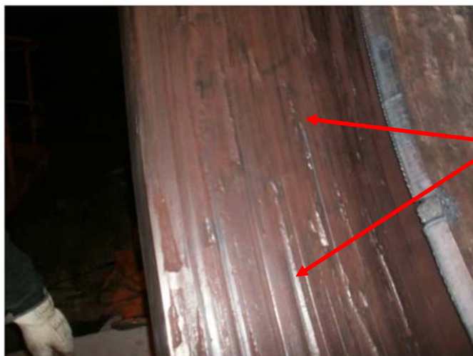
Figure 8 - Tire mounted directly on kiln shell – damage to tire inside diameter when removing from the kiln shell
