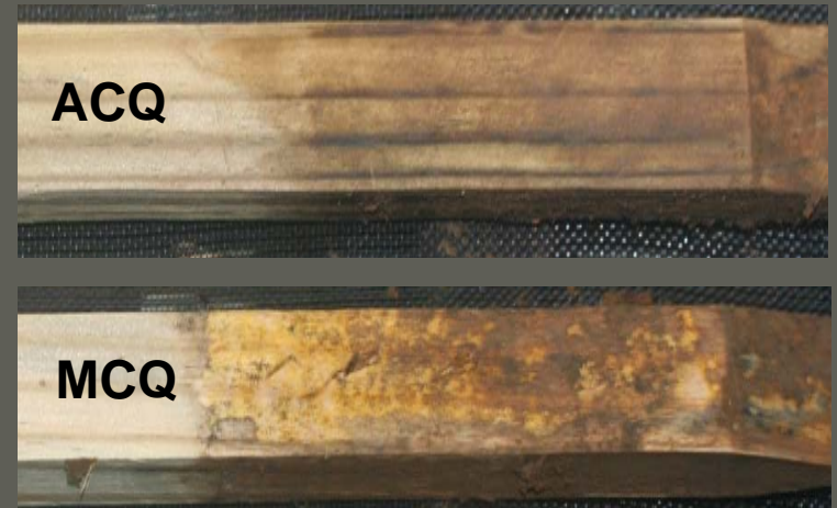
Condition of treated wood stakes after field testing
