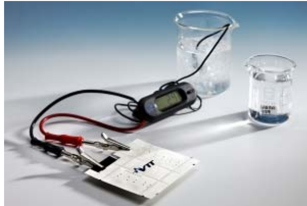
Power source for digital thermometer and Light-Emitting Diode (LED) demonstrated
