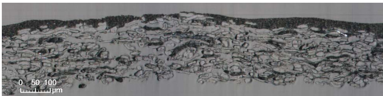
(d) 40% clay in coating color, low base paper porosity.
