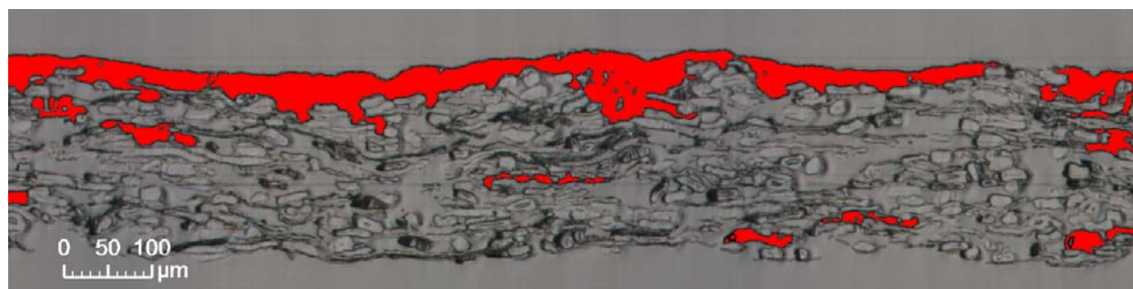
Figure 6: Cross section image (only carbonate containing color, on high porosity base paper region) with detected coating layer highlighted.
