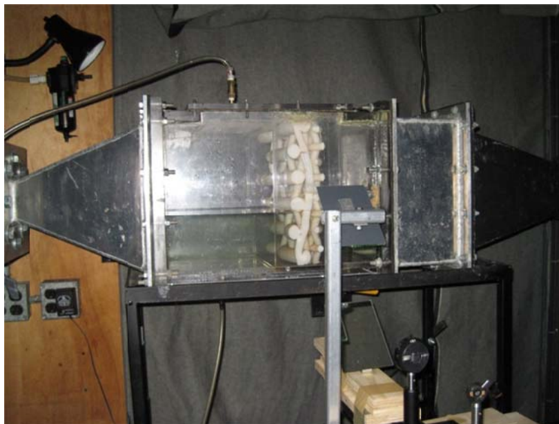
Fig.4. 30cm \times 30cm test section with forming fabric installed
