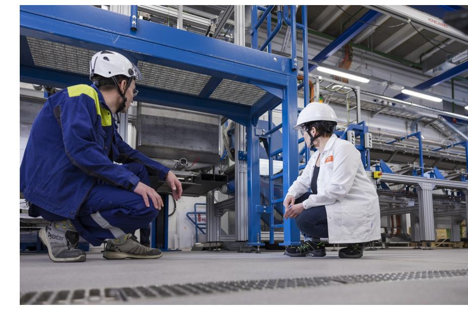
Cellulose films manufacturing line built for technology demonstration. Equipment is designed to produce self-standing regenerated films from cellulose dissolved using various chemistries. Modular concept of the pilot line provides options to partially dissolve fiber webs, in-line impregnation and coating of paper and carton board with the regenerated cellulose film.
