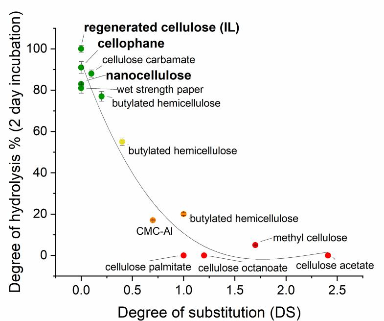
Biodegradation of cellulose-based films by enzymatic hydrolysis in a 2-day incubation. The degree of hydrolysis (%) is presented as the function of the degree of substitution (DS).
