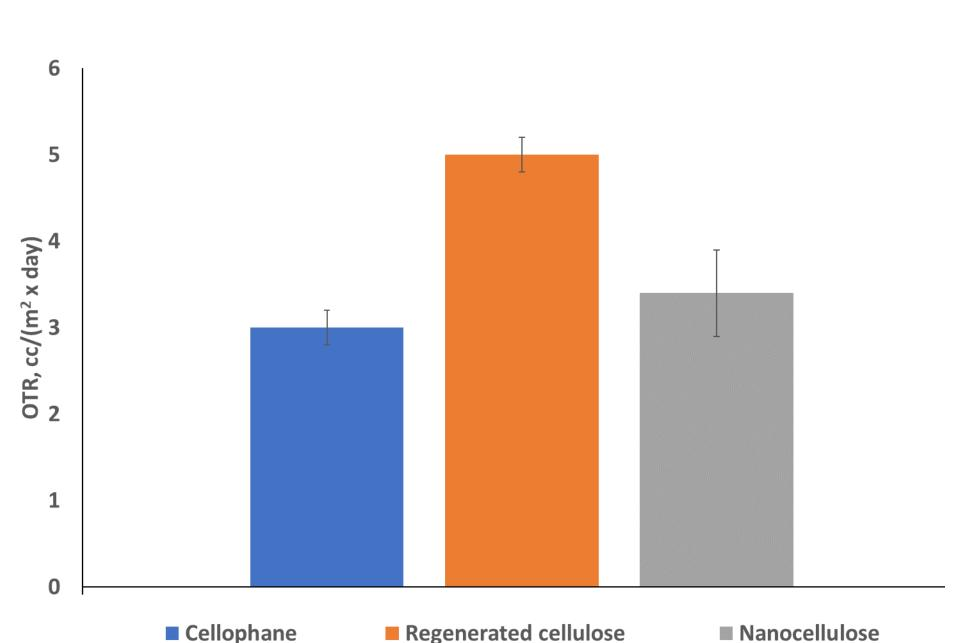
Oxygen transmission rate of different cellulose films measured at 50%RH, 23 °C
