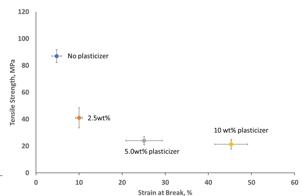
plasticizer consistency **Effect** bath cellulose film (BioCelsol) tensile regenerated strength and strain at break with restricted drying.
