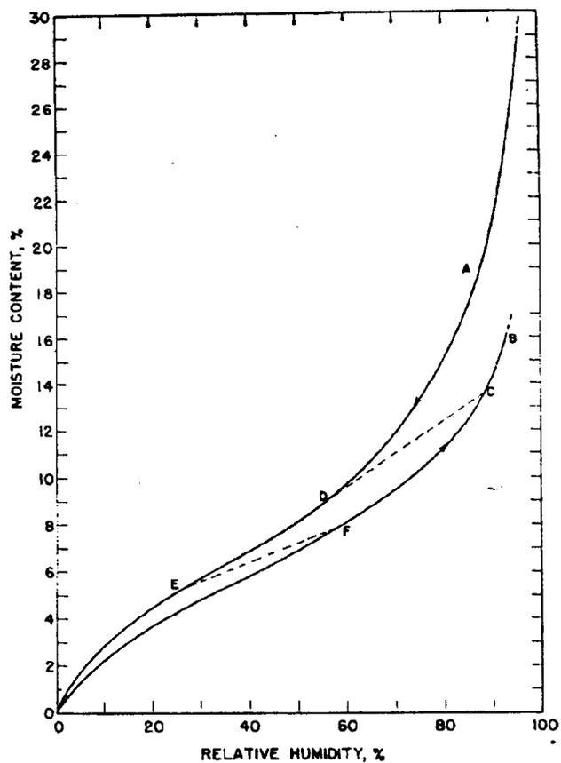
**Fig. 1.** Typical moisture sorption isotherms for pulp and paper. A = desorption curve; B = absorption curve; C = partial adsorption; CD = C followed by desorption to point D; E = partial desorption; EF = E followed by adsorption to point F.
