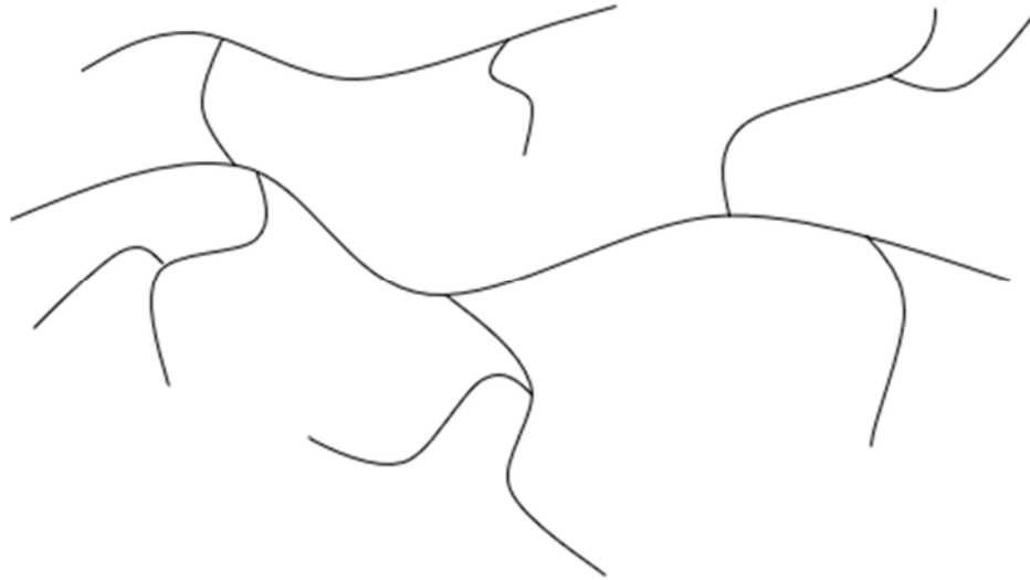
Figure 1. The multibranched structure of LDPE.
