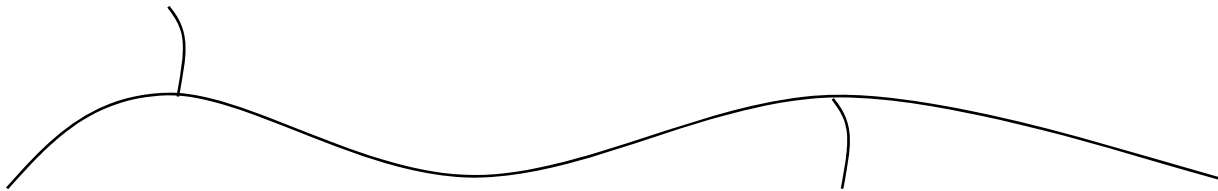
Figure 4. The predominantly linear structure of HDPE.
