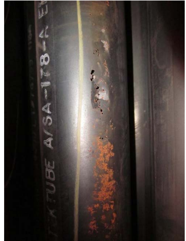
thinned and perforated air heater tube
