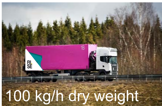
Transportable mobile production plant for nanocellulose CNF pilot in Stockholm
