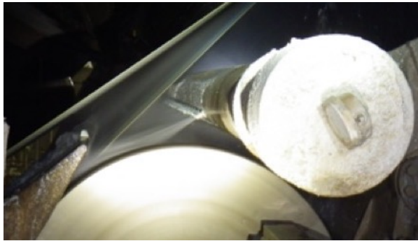
Flooded nip placement: note landing on roll before nip to form puddle
