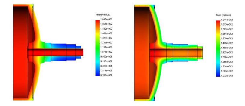
100 psig steam pressure with and without insulating sleeve
