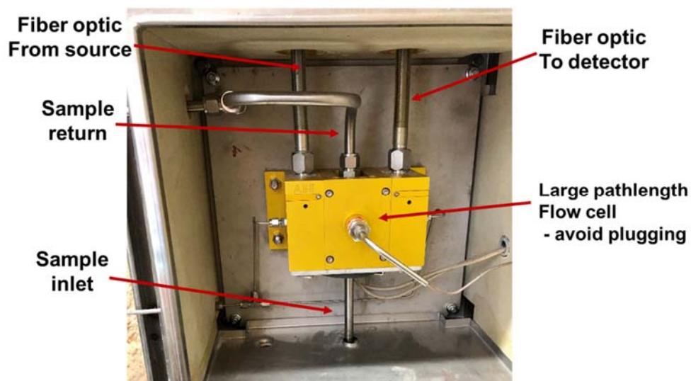
Figure 1: The sample cell of an online analyzer system. Sample flows in from bottom and returns to process. The fiber optic cable brings light to and through the cell and returns to the detector on a second fiber optic cable.
