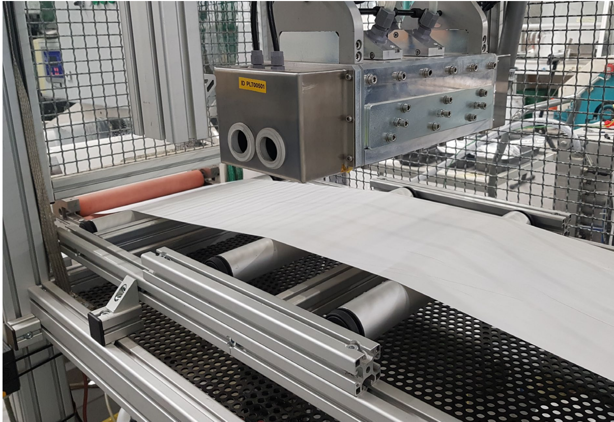
Atmospheric plasma-enhanced chemical vapor deposition R2R pilot unit
