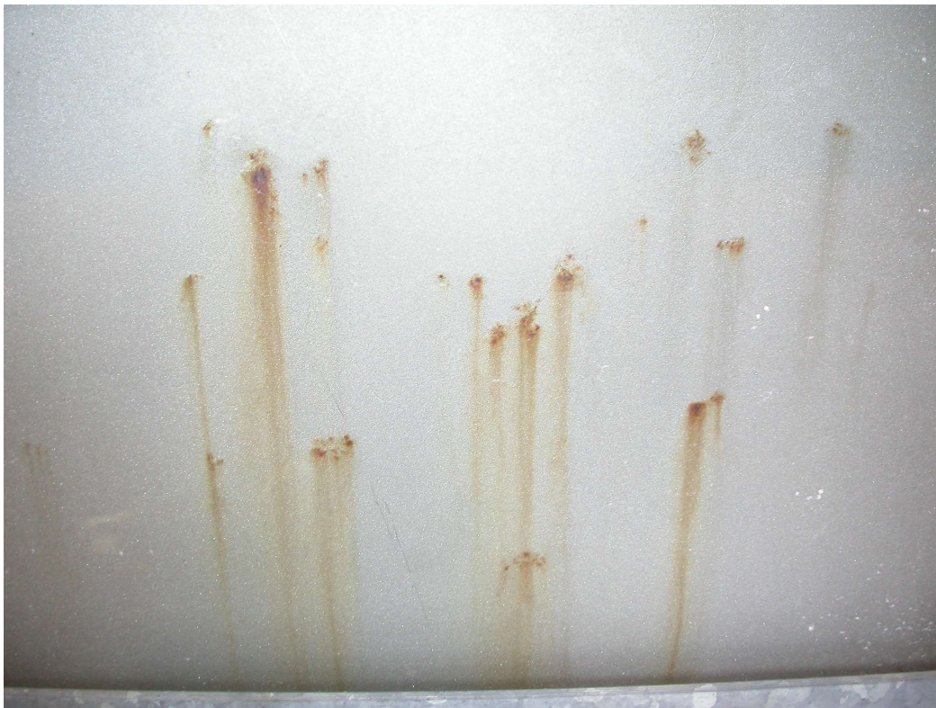
Figure 1. A 317L E/O repulper exposed to D2 filtrate (top) and detail of pitting on the bare trough metal below the inlet pipe (bottom).
