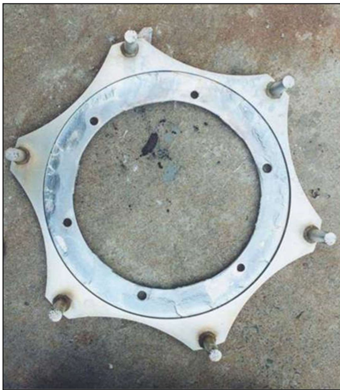
Figure 2. C276 D1 mixer corrosion. The blue coloring is caused by corrosion.
