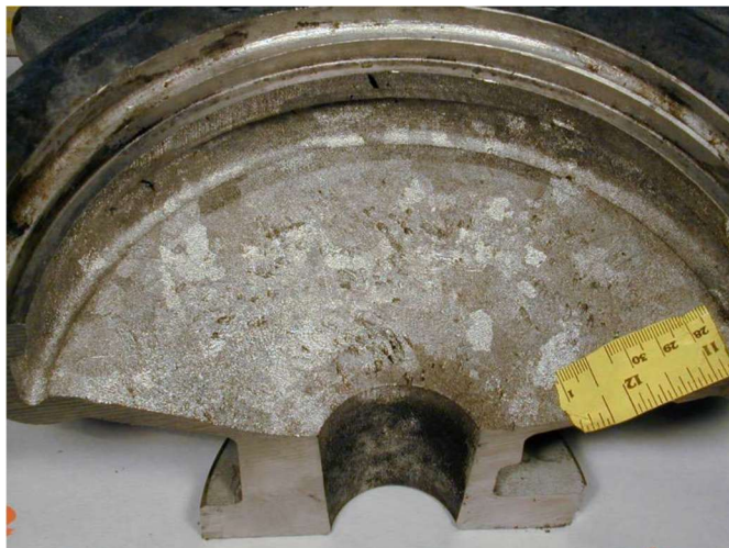
Figure 3. Alloy 20 pump casing corrosion in the form of etching and pitting. The acid concentration was less than 10% acid and the temperature 71 °C (160 °F). High velocity caused it to corrode.
