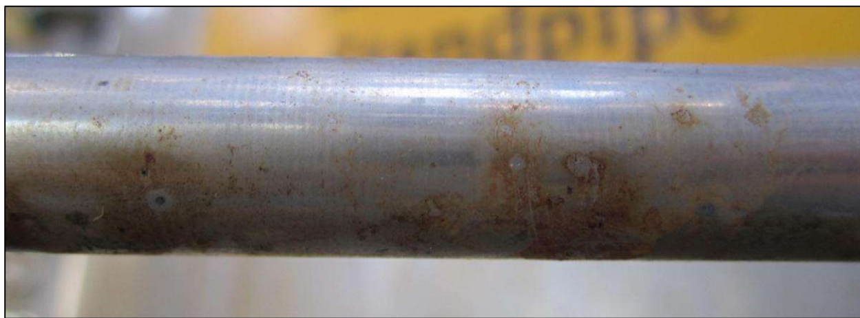
Figure 4. Urea hydrochloride used for pH control pitted 316L piping.
