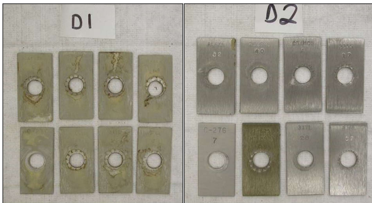
Figure 7. Round 1 coupons after one year of immersion in the D1 and D2 filtrate tanks. The D1 coupons were easily cleaned. No pitting was observed on any of the surfaces.
