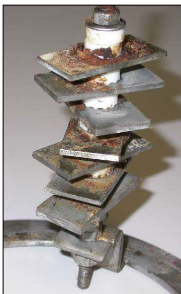
Figure 11. D1 coupons after exposure to the filtrate tank vapor space for two years.
