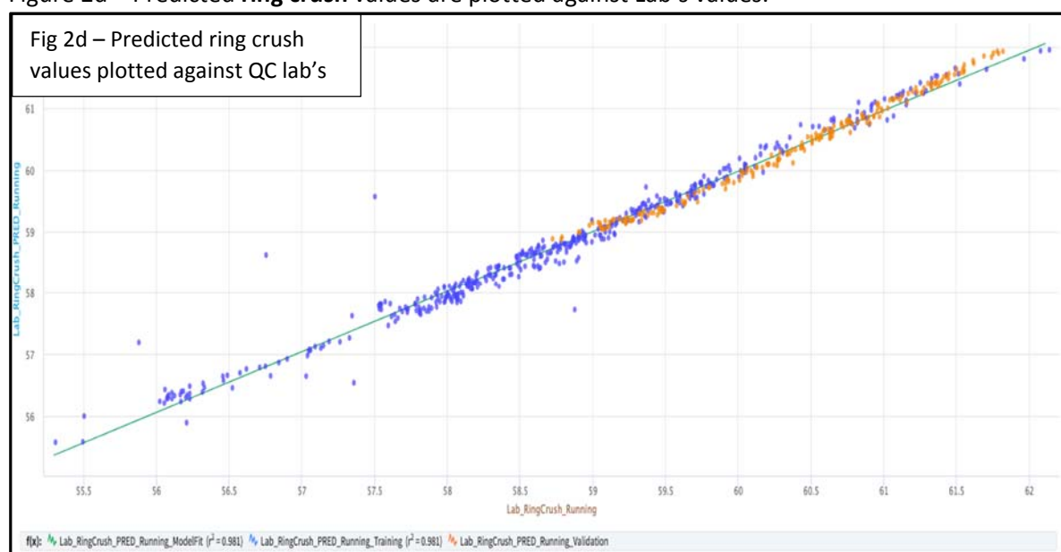
Figure 2d – Predicted ring crush values are plotted against Lab's values.
