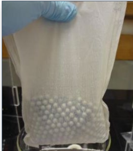
Heat-sealed CF film carrying a load >1.3 kg
