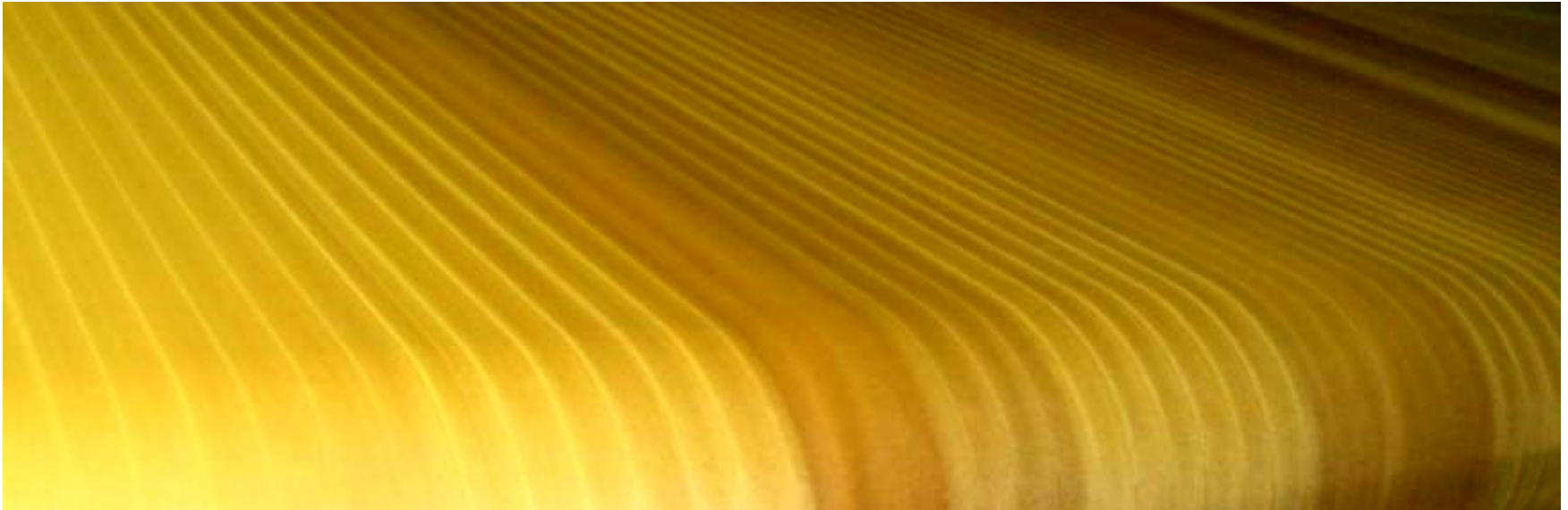
Example of felt streaks (with typical 6" nozzle spacing & 12" oscillator)
