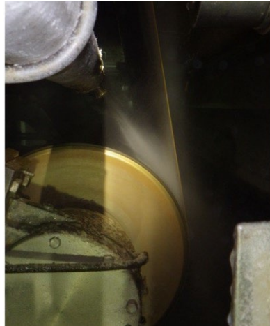
Flooded nip running at reduced volume sufficient for cleaning
