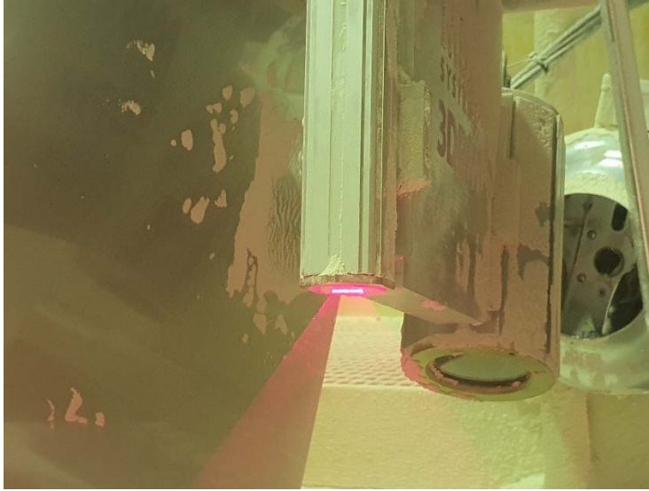
Figure 1. Measurement module showing a laser in the front and a camera in the back.
