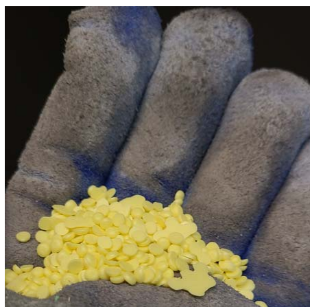
Figure 2 Prilled elemental sulphur
