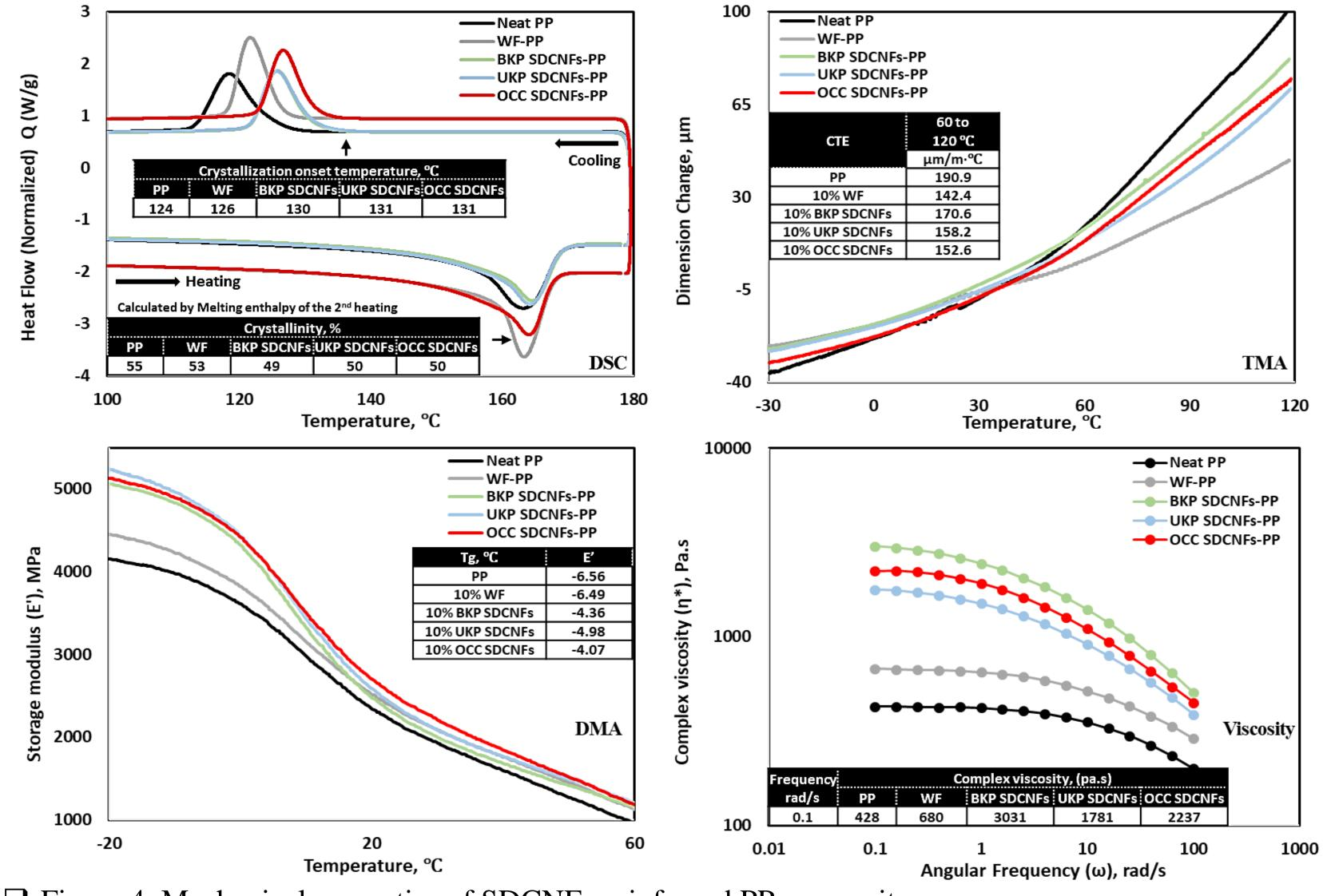
□ Bleached kraft pulp (BKP), unbleached kraft pulp (UKP), and old corrugated cardboard pulp (OCC) were fibrillated to over 90% fines level. Wood flour (WF) was used as a control
